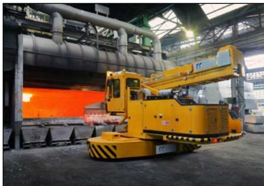
Dross skimming machine in operation at an aluminum melting furnace.
