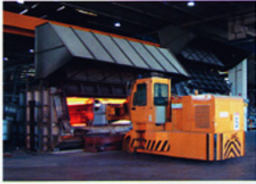
In this illustration, one of the T.T. vehicles is being employed in charging one of Profilglass's holding furnaces
