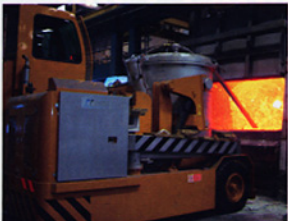
A liquid metal transport vehicle, complete with a discharging device, capable of transporting large quantities of molten metal within the confines of the casthouse
