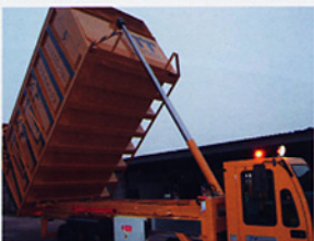
This special truck with a capacity of 50 m 3 was supplied to Profilglass to transport and handle large quantities of aluminium scrap in the client's stockyard
