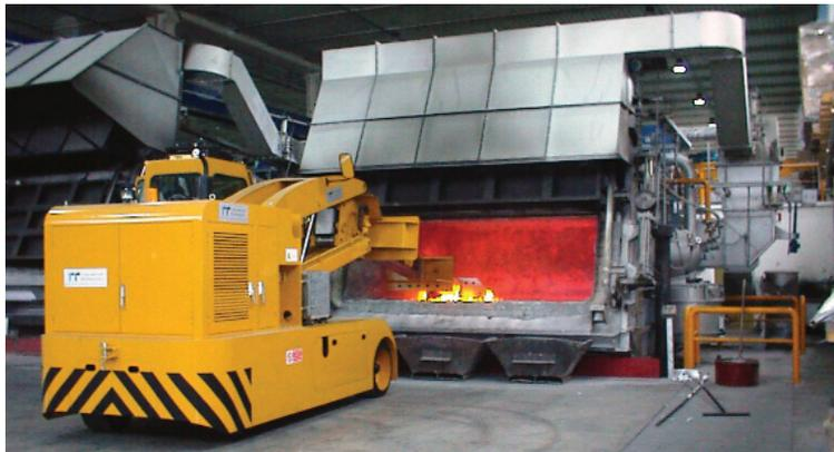
**Cleaning.** The cleaning of the furnace bottom side is performed by a tool flanged to the machine telescopic element.
