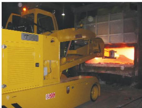
**Unloading of about 4 tonnes of aluminium scrap into the liquid bath without producing splashes. From the driving lifting cab, the operator has complete visibility of this operation.**
