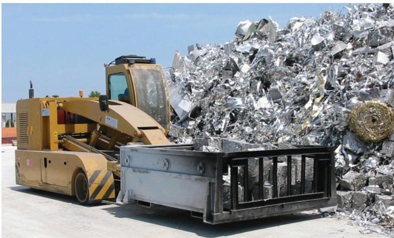
**De-drossing.** As smart alternative option to the use of fork-lift trucks or mechanical shovels, T.T. multifunctional vehicle has a structural stiffness allowing the metal surface de-drossing with the utmost precision as well as the removal of the only dross.
