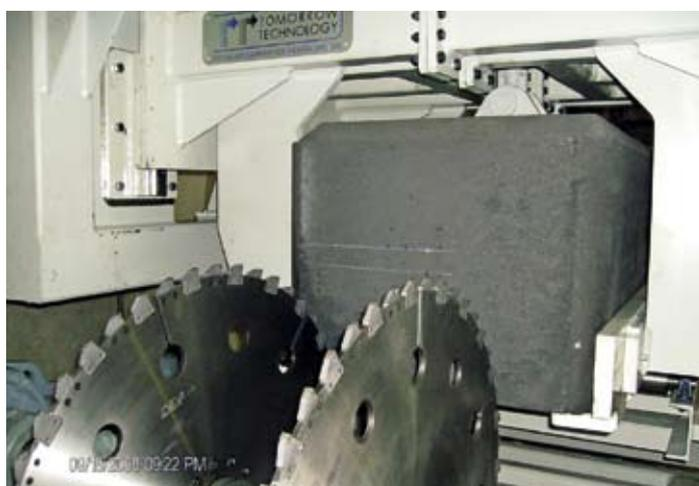
Slotting machine tested in Italy before delivery
