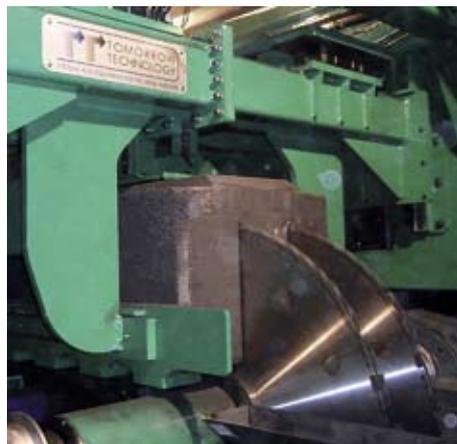
Anodes being cut with two slots 450 mm depth
