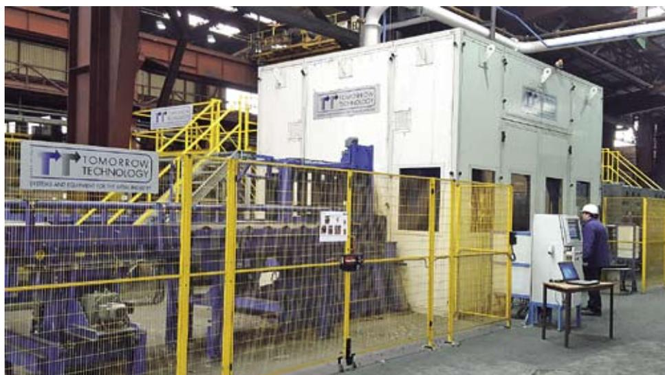
Anodes slotting machine with safety fence
